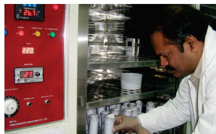
Placing of holding tubes in a climatic chamber maintained at 27 \pm 1^\circ\text{C} and relative humidity of 60-80%
