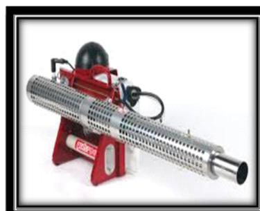
In the second method, petrol is burnt in a specially designed that is constantly supplied with large volume of heated air at low pressure. The formulation is injected into a discharge tube through which air is passing and is emitted as dense fog. This is used in vehicle mounted ones.
