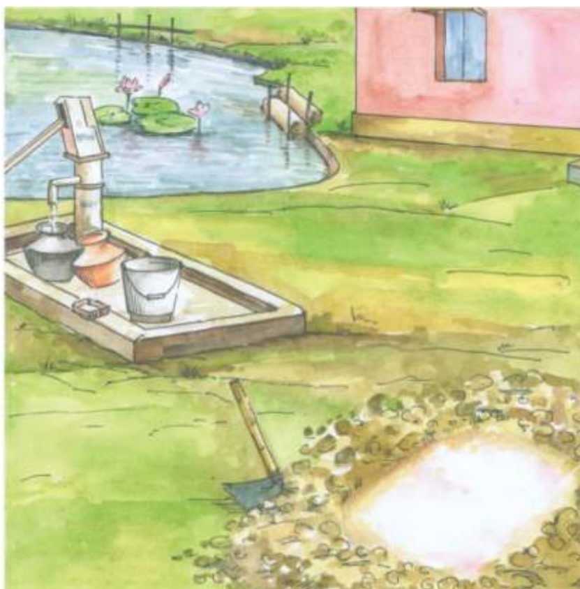
Figure-17: Setting of Soak Pit, Soak pit located on away from water bodies and drinking water source (Source: ECoP, NVBDCP 2012)
